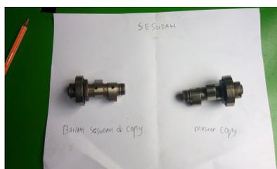
Gambar 11 Sesudah proses grinding
